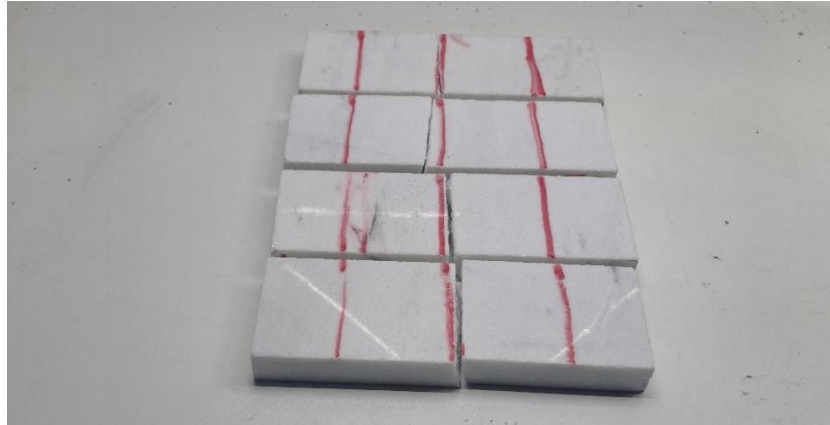
Figure 2 Measurement of flexural strength of Aligudarz crystalline white marble.
